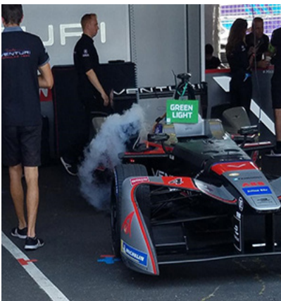
Team uses Dry Ice Cooling Fan on tires during Formula E Races.
